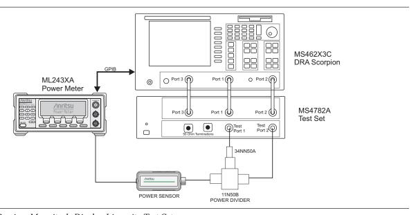
Figure 6-2. Receiver Magnitude Display Linearity Test Setup
