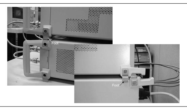
Figure 2-1. ME7840A Component Assembly
