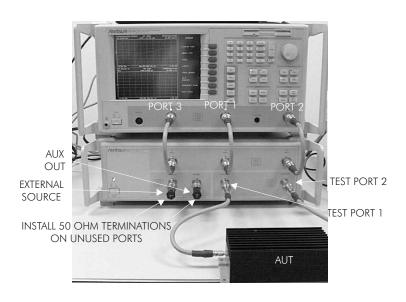
Figure 2-3. ME7840A Front RF Cable Connections (through-line shown between test port 1 and test port 2)
