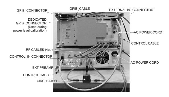
Figure 2-2. ME7840A Rear Cable Connections
