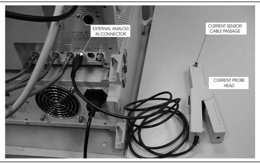
Figure 2-4. Current Probe Connection
