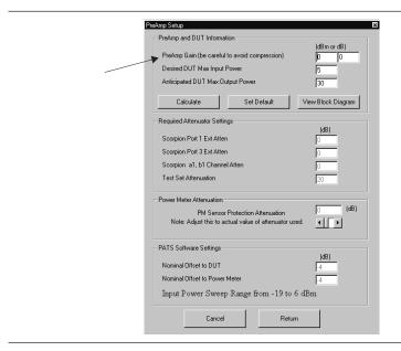
This form helps users set up the ME7840 for calibration. "Set Default" assumes that the user is using the standard MS4782x test set and has a DUT that needs a maximum calibrated input power of +5 dBm and produces a maximum output power of +30 dBm. Think of this form as a spreadsheet. When the user moves to a new field the parameters are "calculated". The user can enter a number and then press the "Calculate" button to make sure the parameters are being calculated.
