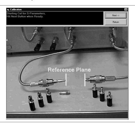
**Step 24.** Connect the Throughline between Test Ports 1 and 2 on the MS4782X Test Set.
