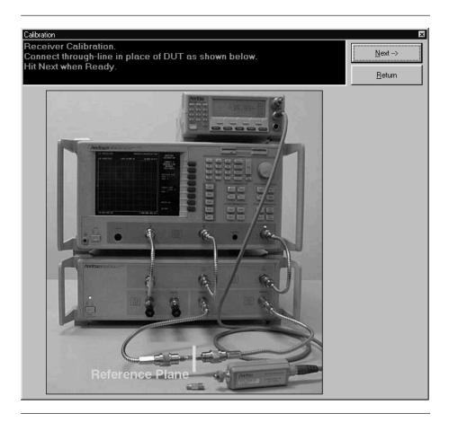
**Step 9.** Press "Next" to perform a receiver calibration. When this calibration finishes, the program returns to the main screen.
