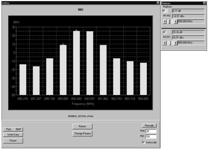
Figure 5-6. Intermodulation Distortion Test Screen
