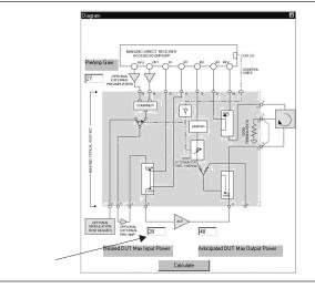
Anticipated DUT Max Output Power: Used to set the maximum output power. Assuming the Max input power is applied to the DUT, what is the expected maximum DUT output power? PA Navigator needs to know this to help set the test set attenuator during calibration and measurement.
