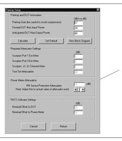
Nominal Offset Power: Note that the value in this box will change as the Power meter attenuation value is changed. Make sure that the value in this box doesn't exceed the specification of the power meter sensor.
