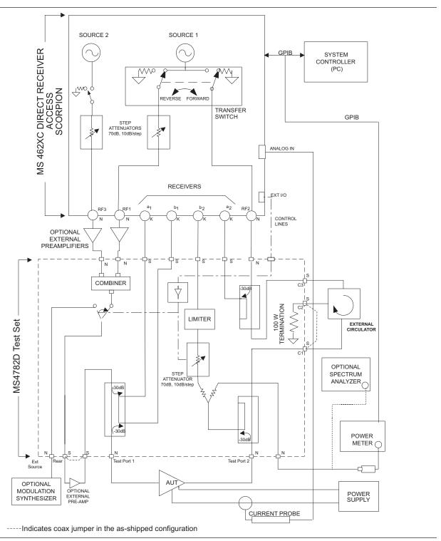
Figure 1-2. Overall Functional Block Diagram of the Basic Power Amplifier Test System (PATS) with MS4782D Test Set
