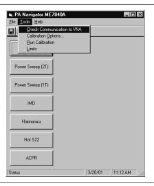
**Step 2.** Click on "Tools" then "Check Communications to VNA" to ensure that the equipment is properly connected to the bus. If so, the following screen will be displayed:
