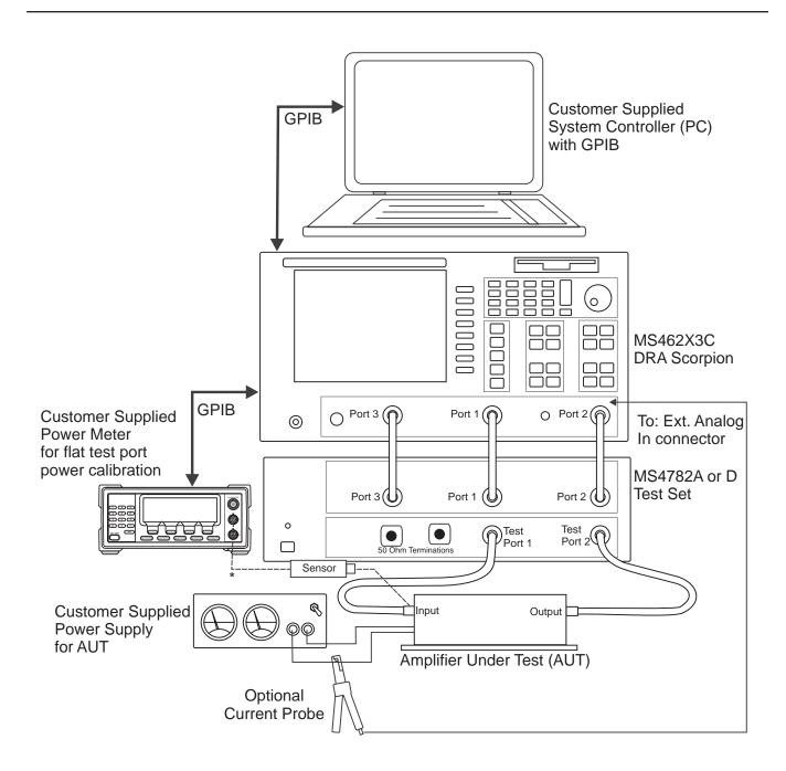
\* Connect when directed by procedure for power calibrations
