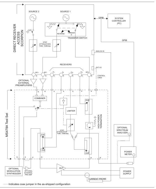
Figure 1-3. Overall Functional Block Diagram of the Option 2 Power Amplifier Test System (PATS) with MS4782A Test Set
