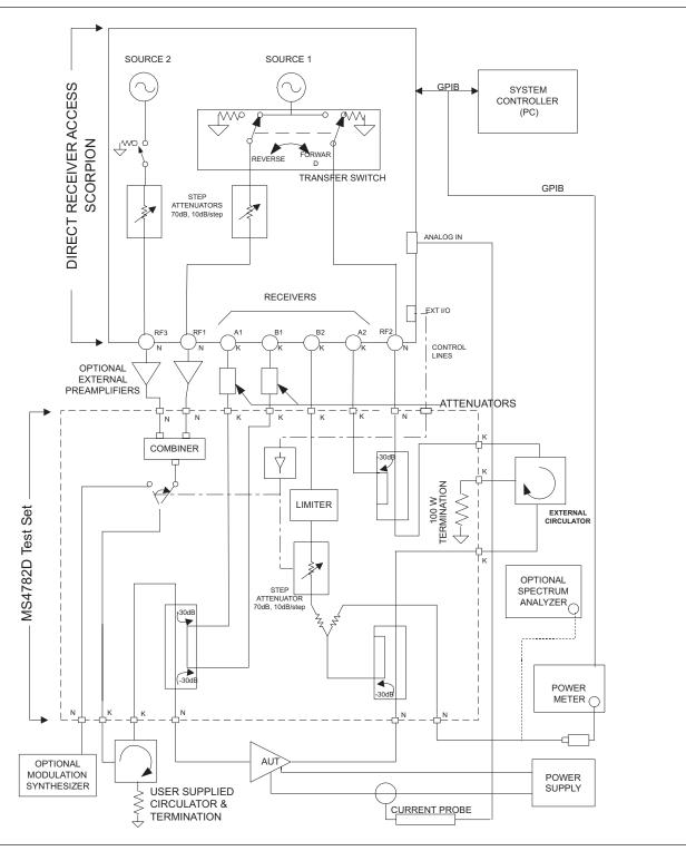
Figure 7-1. MS4782A with External Preamplifiers (Moderate Power)
