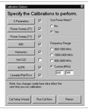
*S Parameters:* Pressing this button brings up the S Parameters screen shown below. Use the drop-down list arrow keys to display parameter selections.
