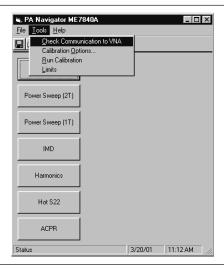
a. Check Communications to VNA: Runs a test to check that the VNA communicates with the PC. Run this option first to ensure that the PATS setup is correct and functioning properly. If so, a dialog box appears like that shown below.
