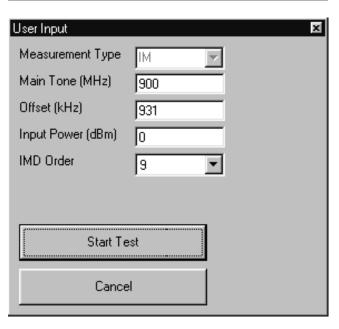
Select **Start Test**. Observe that the test screen (Figure 5-6) appears.
