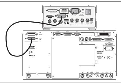
Figure 6-1. ML2430A Series Power Meter GPIB connection to the MS462XX Vector Network Measurement System
