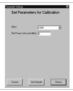
Cal Setup Wizard: Provides forms (shown on next page) that will automatically set some parameters, like nominal offset, and suggest attenuators to add to the calibration and measurement setup.Run the Cal Setup Wizard before running the calibration.
