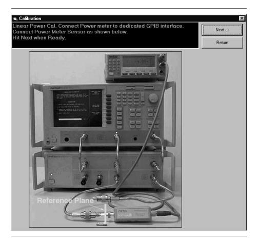
**Step 6.** Before hitting the "Next" button, connect the power meter to at the point where power enters the device-under-test (AUT), which becomes the power reference plane as shown in the prompt.
